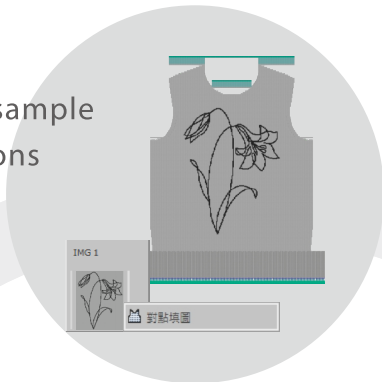
Fill selected pattern by fill-point indicated in the knit specification
